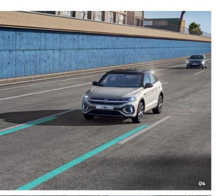
**03 Front Assist** emergency braking system with pedestrian detection can alert you to critical situations involving pedestrians and other vehicles and even apply the brake automatically in emergencies.
